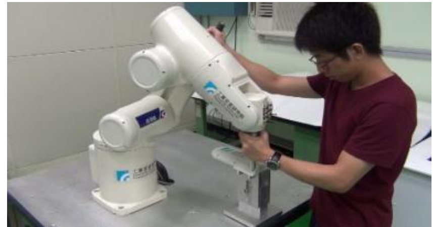
Teaching a trajectory following task on a surface
