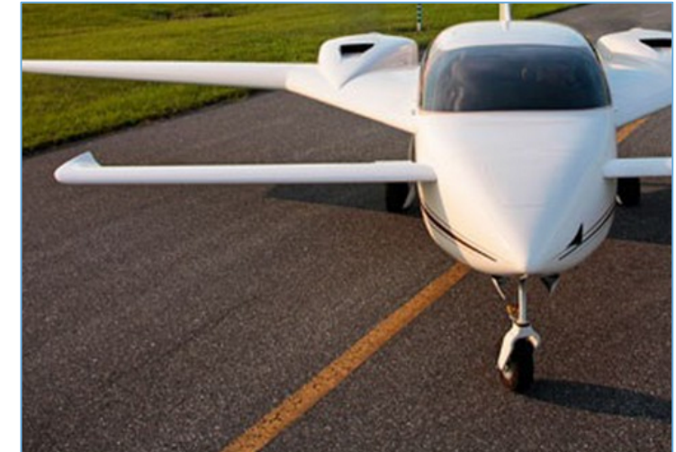
Hempearth's plane is made of hemp-and-resin panels, a sustainable and lighter alternative to traditional materials.
