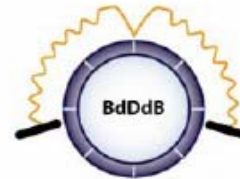
Barriers with small detents and large center detent
