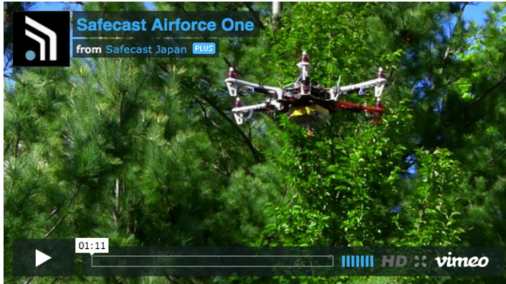
The above video is a hexacopter with an onboard bGeigie Nano taking radiation readings in flight and broadcasting live via wifi. It's the result of the just finished week long Safecast hackathon that just took place in Cambridge, MA.
